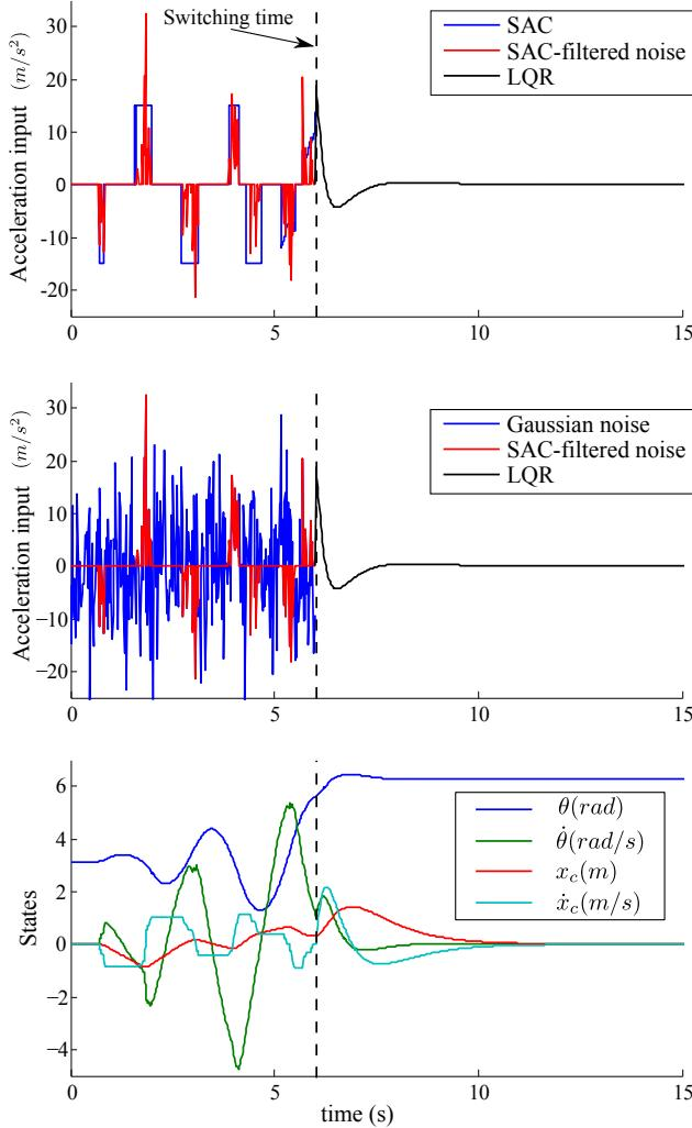
Fig. 3. Sample simulation for the cart pendulum system. The top two plots demonstrate the similarity of our controller/filter with Maxwell's demon; SAC as a filter rejects noise samples that would otherwise lead the system to a different control direction.
