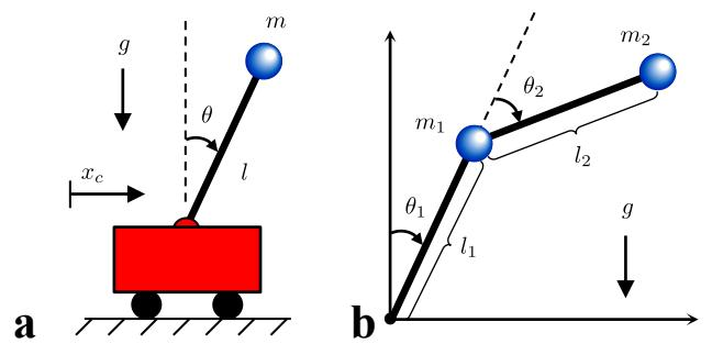
Fig. 2. Schematic of the cart pendulum system (a) and the acrobot/pendubot (b).
