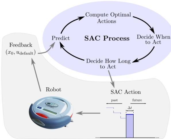
Fig. 1. An overview of the SAC control process.
